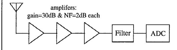
amplified using 3 amplifiers with a nominal gain of 30 dB and noise figure of 2 dB. A total of 92 dB of gain was measured from three amplifiers combined. The filter following the amplifier chain has an insertion loss of 3.2 dB and 3 dB and 30 dB bandwidths of 3.4 MHz and 10.3 MHz, respectively. It is difficult to build a filter with a narrower bandwidth, because of the relatively high center frequency. The filter dimension is 3x6x14 cm<sup>3</sup>.
